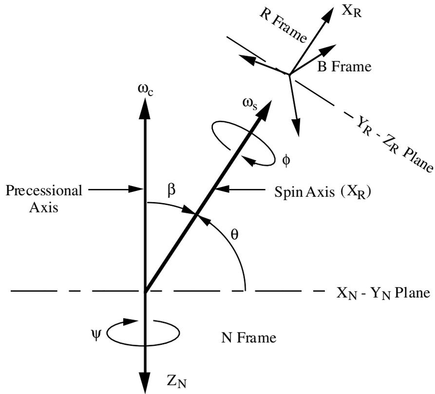
Figure 1 - SPIN-CONE Geometry
