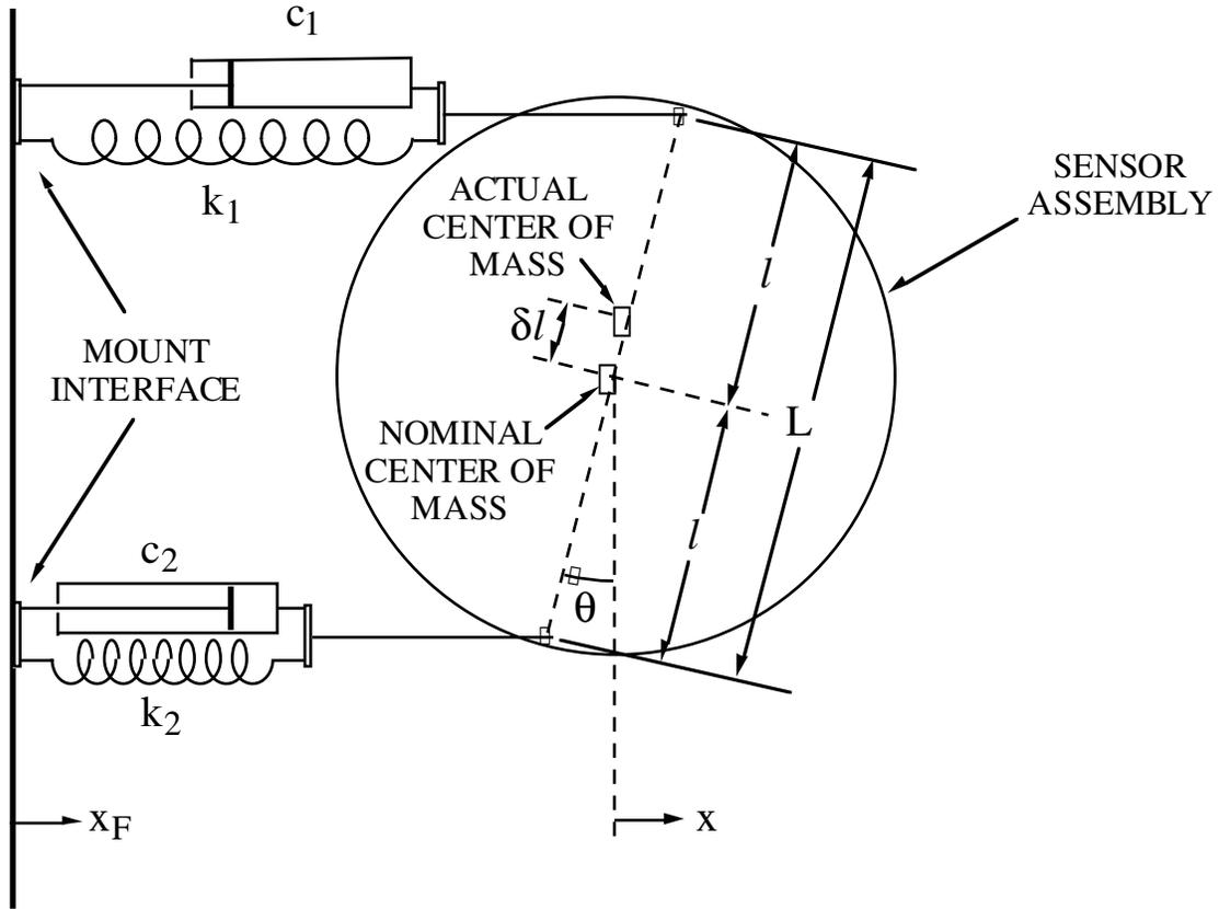
**Figure 3 - Simplified Sensor Assembly Dynamic Response Model**
